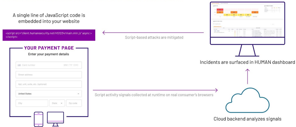
Figure 8: The HUMAN sensor deploys with a single line of code to entities' websites, running on every consumer's browser, to provide complete visibility and control of script behavior and HTTP headers.
